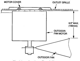
Fig.24 — Outdoor-Fan Adjustment
